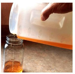
Pour the oil from the Clean Oil Container and then reassemble the unit.
